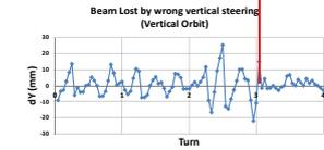
Beam loss caused by Vertical Oscillation after 3 turns. Change in sum of 4 electrodes signals clearly exhibits the position of beam loss. This case: in B2 bending duct
